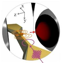
employed to measure the faint interaction of a nanowire with a single spin qubit [4,5]. In the envisioned experiment, a single NV spin qubit hosted in a diamond nanocrystal attached to the vibrating extremity of a nanowire and coupled to its vibration by means of a strong magnetic field gradient. In analogy to the historical Stern and Gerlach experiment, the resulting strong hybrid spin-mechanical interaction will be used to perform a mechanical readout of the single spin quantum state.
